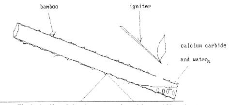
Fig. 2: A self-made bamboo canon using calcium carbide and water
