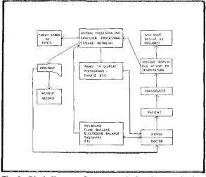
Fig. 2 Block diagram of a computerised patient monitoring system with facilities for automatic and manual data entry.  $^4$
